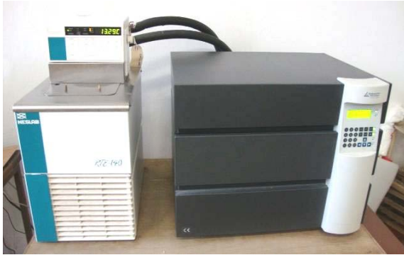
Fig. 3 Apparatus Holometrix 2300 for determination of thermal conductivity
