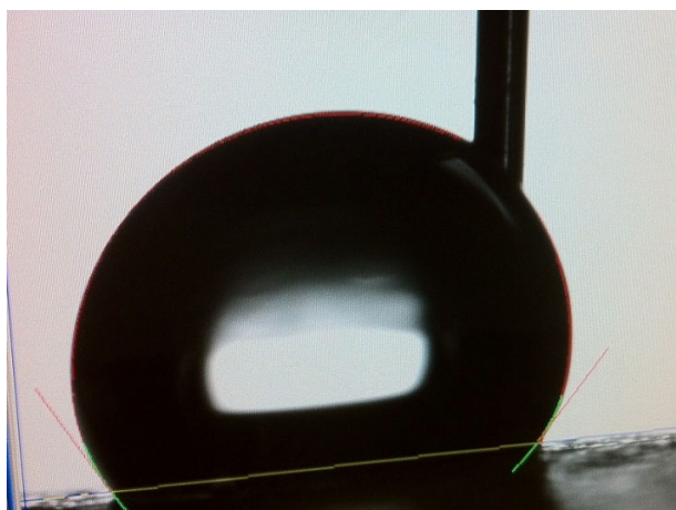
Fig. 5 Equilibrium state of a distilled water droplet on a flat-sheet membrane active layer (PTFE)
