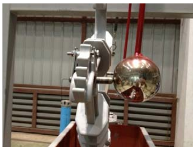
Fig. 3 Voltage Energized via Stainless Rod and Stainless Sphere
