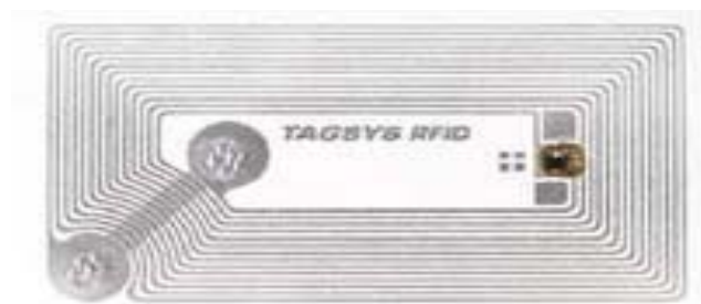
Fig. 2 RFID Tag for Pharmaceutical Industry
