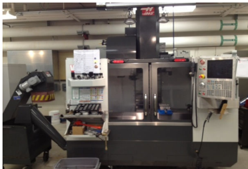
Fig. 3 CNC HAAS Vertical Machining Center, Model VF2TR
