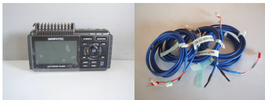
Fig. 4 Graphtec data loggers and thermocouple wires
