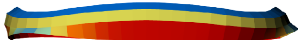
Fig. 8 Elevation – Visualisation of membrane slopes – Snow applies on blue panels (slope is less than 30°)
