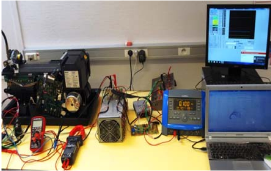
Fig. 7 Photo of the test bench of the electronic load with the Ballard Nexa™ PEM fuel cell
