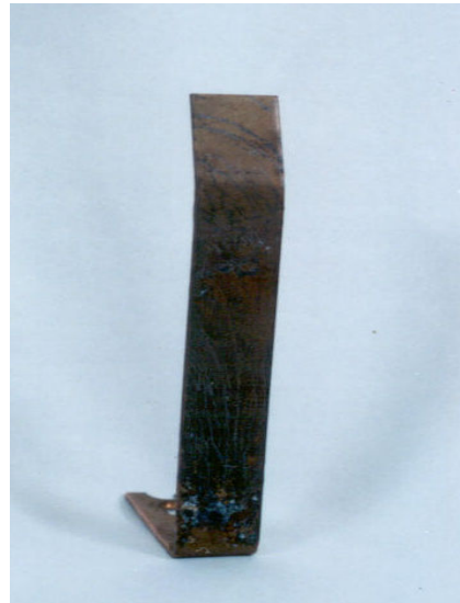
Fig. 6 The photograph of a test electrode copper of 1 mm thickness
