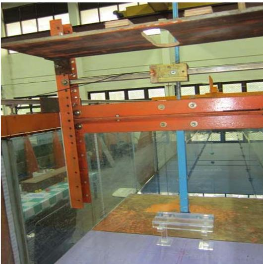
Fig. 9 Photo of the bridge model installed inside the flume
