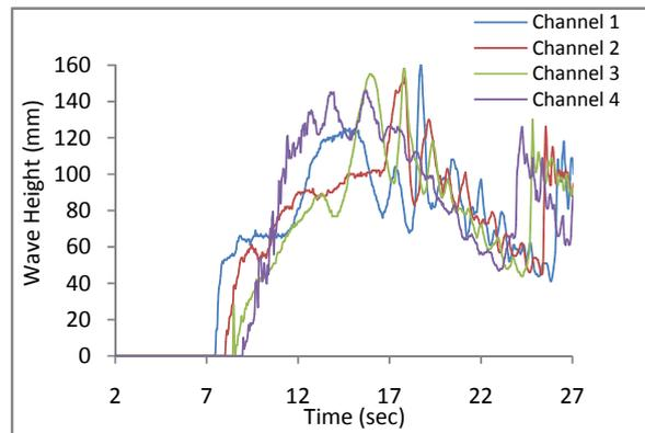
Fig. 11 Measured time histories of tsunami wave height
