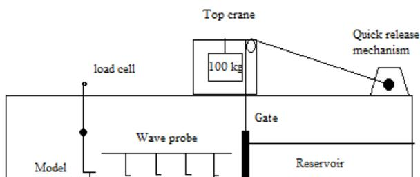
Fig. 6 Experimental Setup
