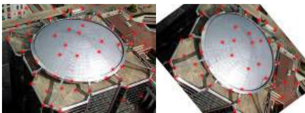
Fig. 4 Image processing using siftmatching
