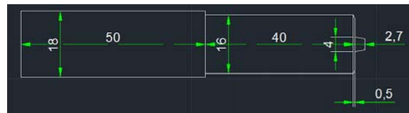
Fig. 6 Friction stir welding taper cylindrical tool
