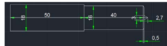
Fig. 7 Friction stir welding triangular tool
