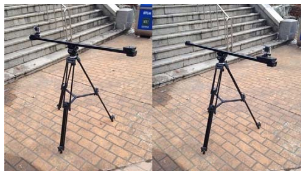
Fig. 2 Stereo video acquisition using Gopro
