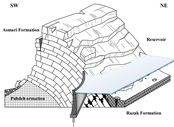
Fig. 9 Block diagram of the Salman Farsi dam foundation rocks on the northern flank of the Chagal Anticline. Showing dam body/cut off curtain, reservoir area and distribution of the Pabdeh (marl), Asmari (karstic limestone) and Razak (gypsum) formations
