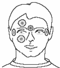
Fig. 1 The electrode positions around eyes for horizontal and vertical motion
