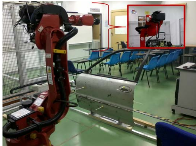
Fig. 1 Experimental setup showing the work piece (car door) and the end effector where a camera were installed marked in the small box in the figure
