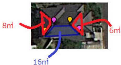
Fig. 3 Measurement of the area of the roof
