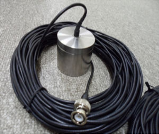
Fig. 5 Ultrasonic Sensor after waterproof
