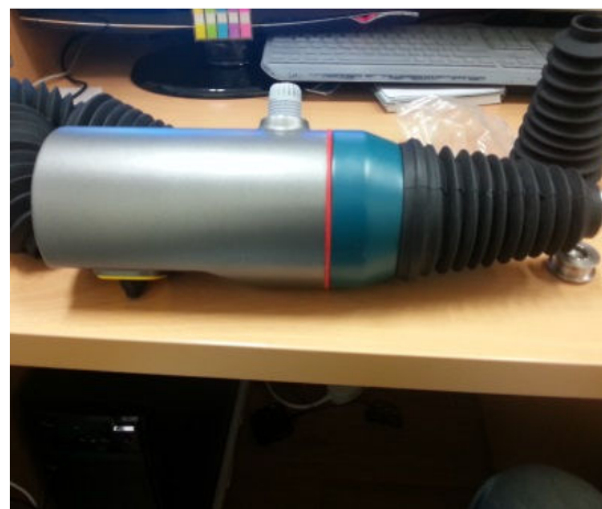
Fig. 2 Schmidt hammer after waterproof
