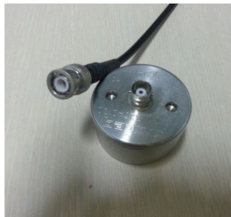
Fig. 4 Ultrasonic Sensor before waterproof
