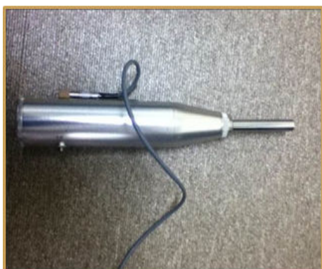
Fig. 1 Schmidt hammer before waterproof
