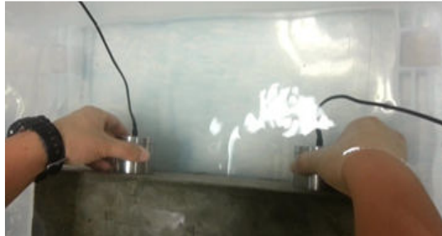
Fig. 7 Ultrasonic pulse velocity test in under water condition
