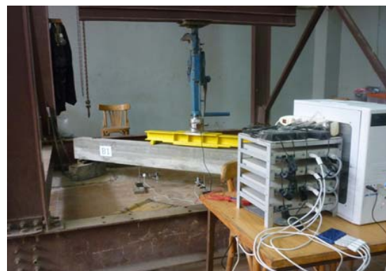
Fig. 4 Splice beam prior to testing
