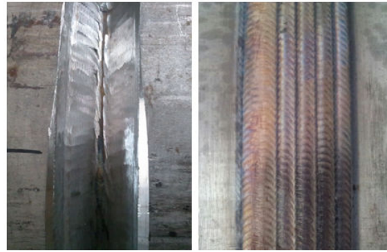
Fig. 9 Before and after welding quality of Duplex steel
