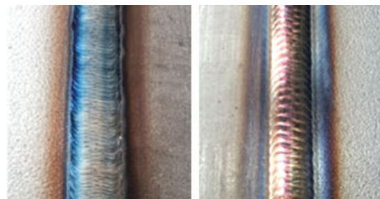
Fig. 7 Welding quality of manual welding vs. automatic welding
