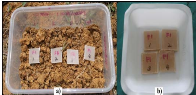
Fig. 7 Sample of LDPE/TS: 70/30 a) before and b) after the soil burial test
