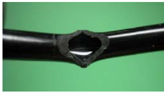
Fig. 2 Deformation of the CSDS during bending
