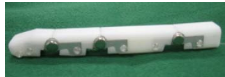
Fig. 11 Prototype of the robot finger incorporating CSDS
