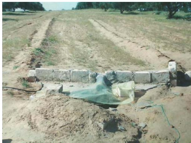
Fig. 2 The station in the field for measuring erosion and surface runoff
