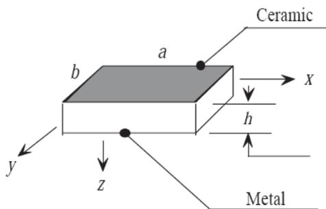
Fig. 3 Schematic diagram and dimension of plate
