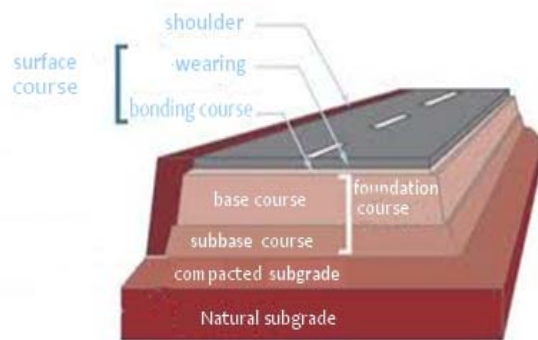
Fig. 7 A cross section of a roadway
