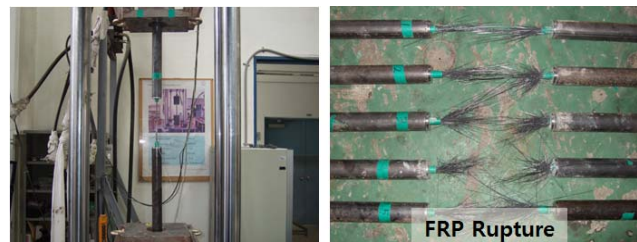
Fig. 5 View of tensile test and failure pattern
