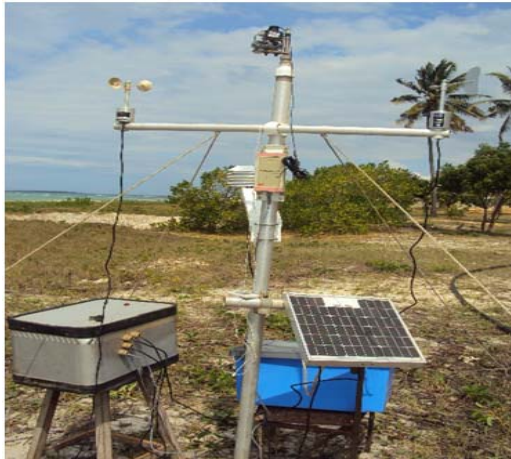
Fig. 2 Experimental set up for the measurement of wind speed and direction
