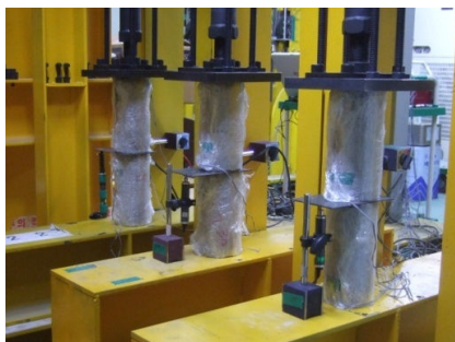
Fig. 4 Creep test of base course mixes
