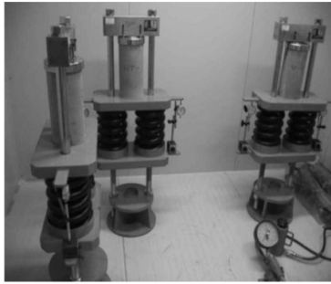
Fig. 2 Hydraulic creep test device
