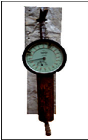
Fig. 4 Disposition of test pieces when testing shrinkage
