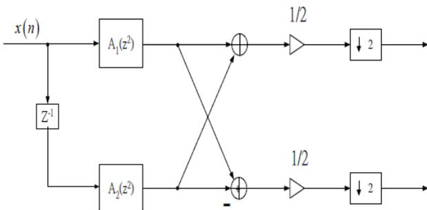
Fig. 2 The analysis system of the DC-based QMF bank
