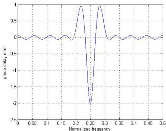
Fig. 9 Group delay error of the filter bank using the method of [11]
