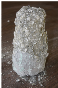
Fig. 2 Decomposition of a specimen exposed to 900°C
