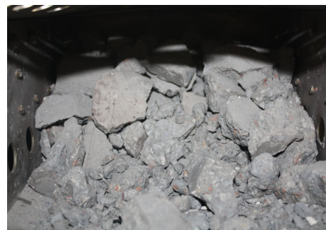
Fig. 3 Explosive spalling at 425°C on N series
