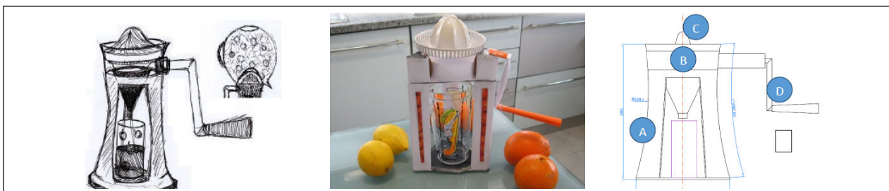
Fig. 6 From concept, in the left, to a looks like prototype in the centre and to detail design, in the right. Adapted from [24]
