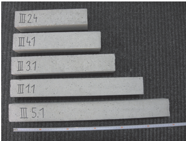
Fig. 7. Five different lengths of concrete samples.
