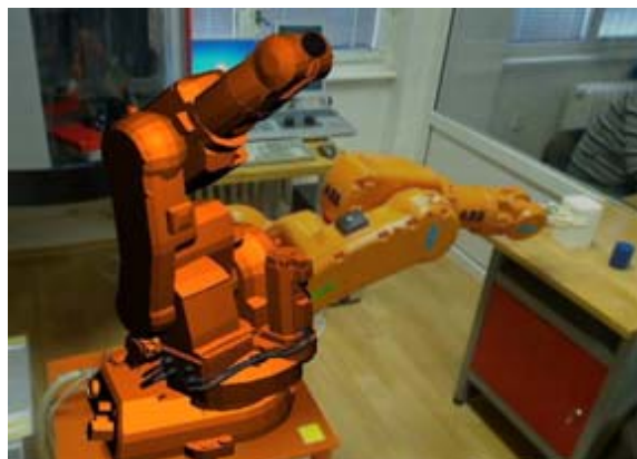
Fig. 4 Virtual model of robot in real environment
