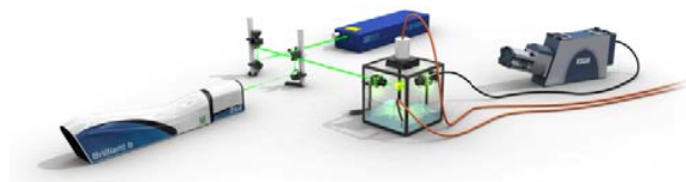
Fig. 1 LIBS system arrangement employing water jet
