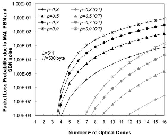
Fig. 4 Packet Loss Probability due to MAI and beat noise as a function of the number  $F$  of Optical Codes for  $L=511$ ,  $H=500$  byte and  $p$  varying from 0,3 to 0,9. The curves labeled with OT report the results when the Optimized Threshold is used
