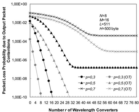
Fig. 5 Packet Loss Probability  $P_{loss}^{opc}$  due to output packet contentions as a function of the number  $r$  of used WCs. The curves labeled with OT report the results when the Optimized Threshold is used
