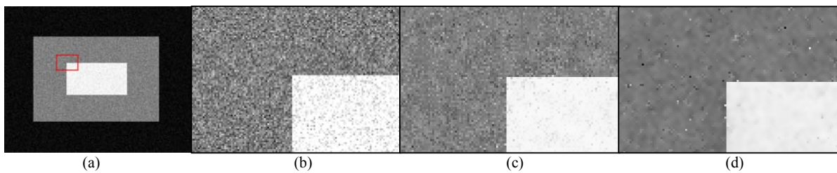
Fig.6 (a) the original test image; (b) local details from (a) within the small red frame; (c) the result by BF (one iteration), the time cost is 1.80s, SNR=17.3, the kernel size is 33 \times 33 and (\sigma_c, \sigma_s) = (2.5, 31.62) ; (d) the result by MGBF, the time cost is 0.27s, SNR=46.8, (\sigma_c, \sigma_s) = (2.5, 10) .
