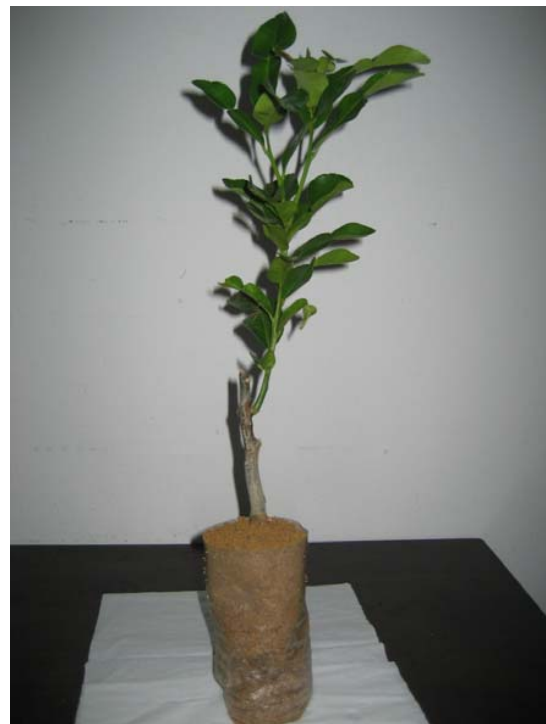
Fig. 9 BioPot from corn husk composite film
