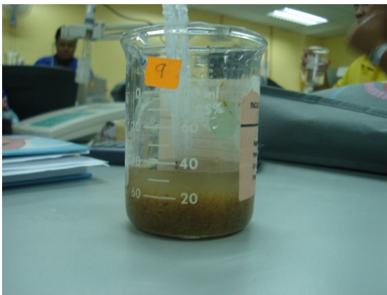
Fig. 2 Chemical treatment of corn husk
