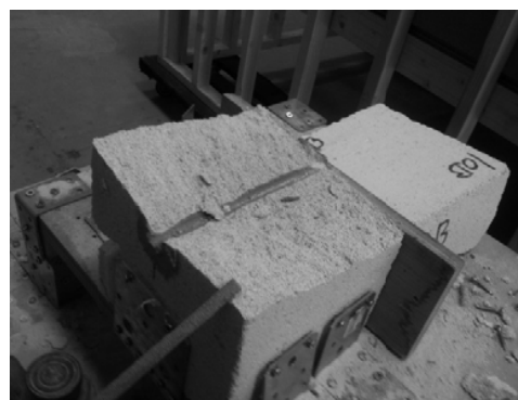
Fig. 3 Total spalling, crushing in front of reinforcement
