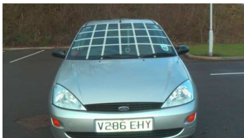
Fig. 4 Marking out windscreen cells
