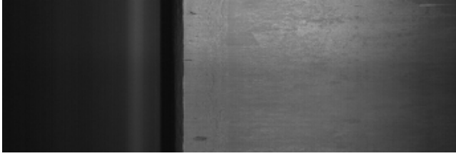
Fig. 2 Surface image of a steel plate with seam cracks
