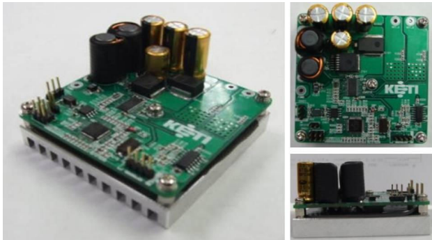
Fig. 9. Photos of VVA drive.
