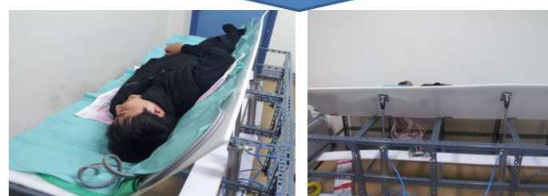
Fig. 4 Position change using air cylinder
