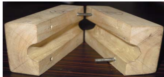
Fig.2. Split wooden mould
