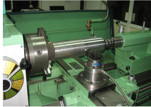
Fig. 4 Photo of lathe fitted with inserts
