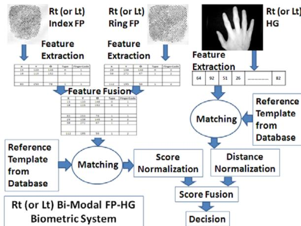
Fig. 17 Schematic for Rt-HG-FP (or Lt-HG-FP) MMBS
