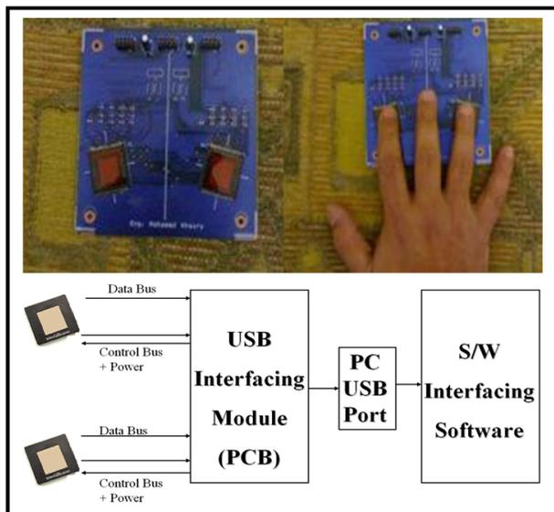
Fig. 2. Two FP capacitance sensors installed on a single PCB to acquire both Index and Ring FP (top) and its USB interface (bottom)
