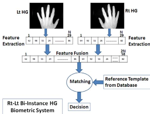
Fig. 6 Rt-Lt-HG (Feature-Level fusion) bi-instance biometric system schematic
