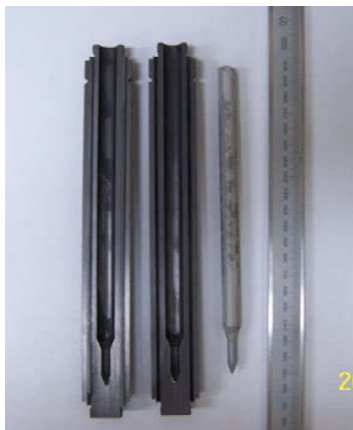
Fig. 2 Graphite mould used in this study and as-grown crystal of pure Mg
