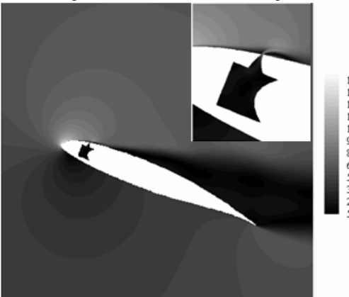
Fig. 9 Contour plots of velocity magnitude (m/s) over an airfoil at angle of attack, \alpha = 22^\circ , blowing-out segment
