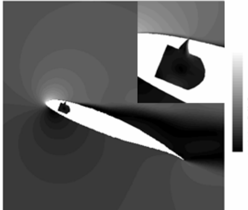
Fig. 8 Contour plots of velocity magnitude (m/s) over an airfoil at angle of attack, \alpha = 22^\circ , suction segment
