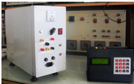
Fig. 3 Electrical and Controller unit of PEF set
