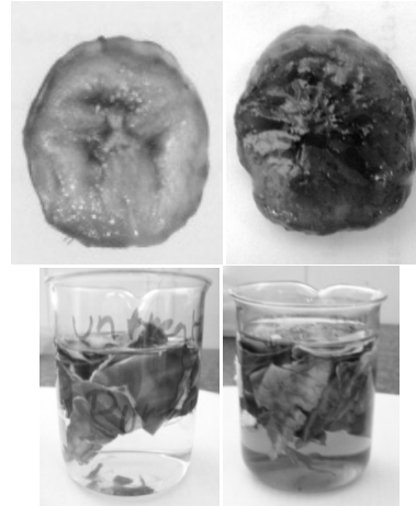
Fig. 6 the effect of 1000 pulse on the material (5kV, 100 \mu s, purple cabbage and banana after 24 hour) Left sample without PEF and right sample with pulse exertion
