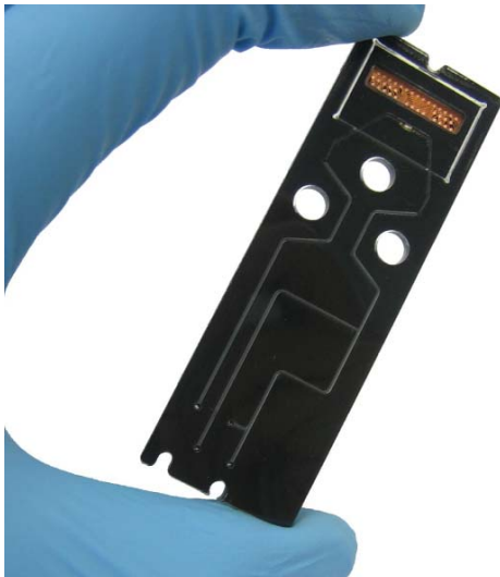
Fig. 5 Fabricated flow cell with integrated sensor package; A homogeneous bond was observed, without any indication of thermal decomposition
